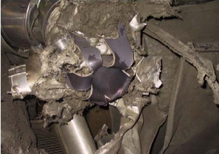
picture 2-2: Brunsbuettel ruptured tube (HIRSCH 2005)
